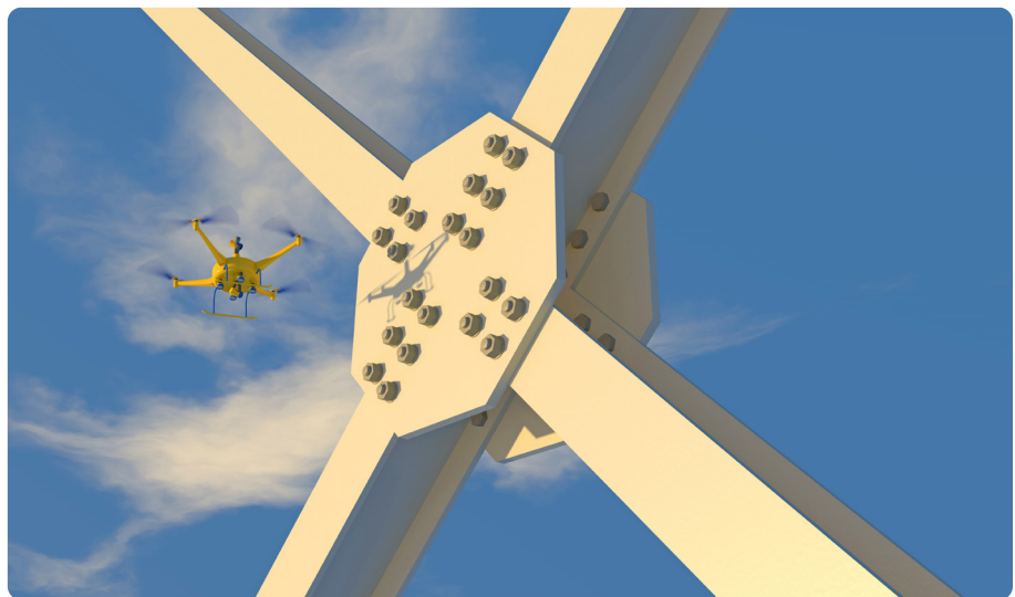
FIGURE 2. QUADCOPTER DRONE INSPECTING A BRIDGE
